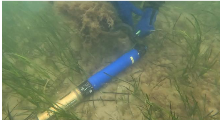
Figure 5: Water quality monitor being deployed in Studland Bay (image: Ken Collins)
