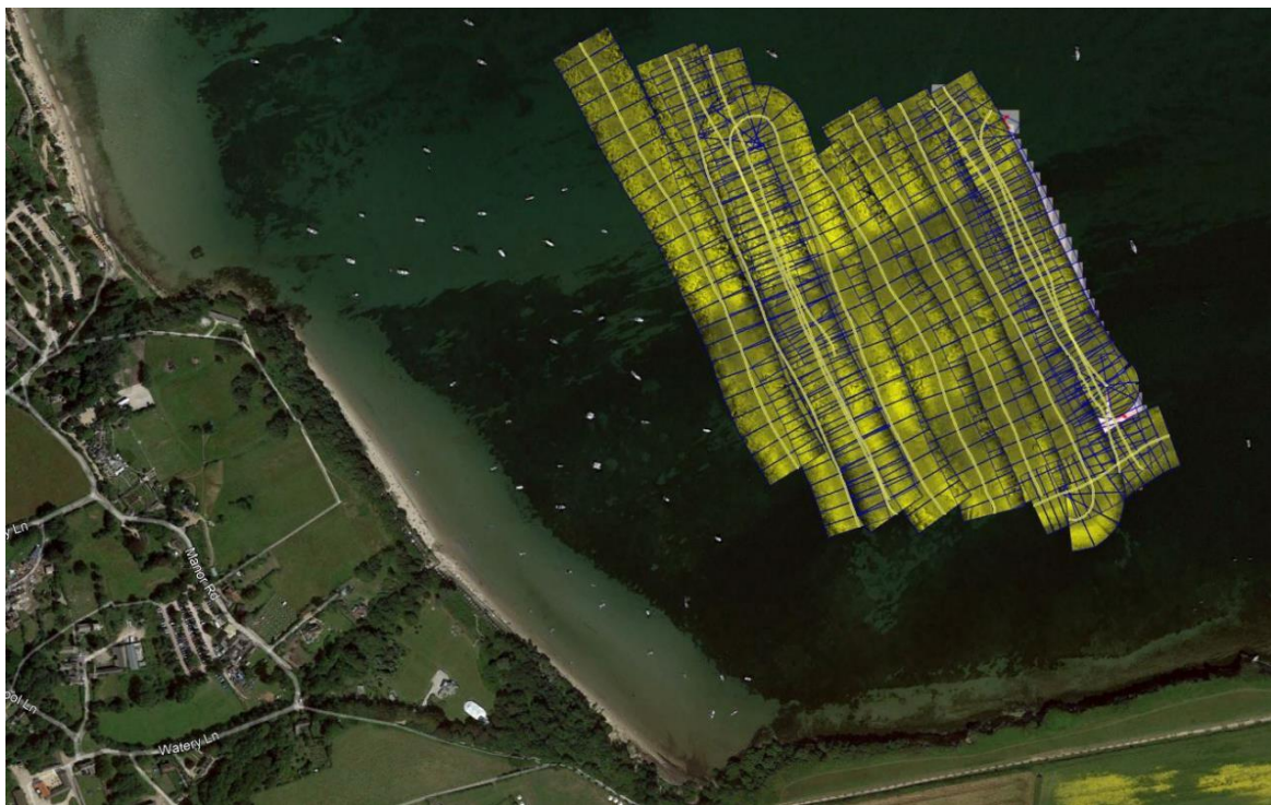
Figure 1: Side-scan sonar data is used to monitor the extent of the seagrass beds and the size of anchor scars (Image - Ken Collins).
